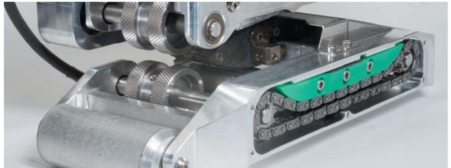
The welder is equipped with a drive system that does not require any maintenance and ensures fast and reliable “weld-wise” movement throughout the process, including for foils up to 3.5 mm (4 mm) thick, at a maximum speed of 6.00 m/min.
